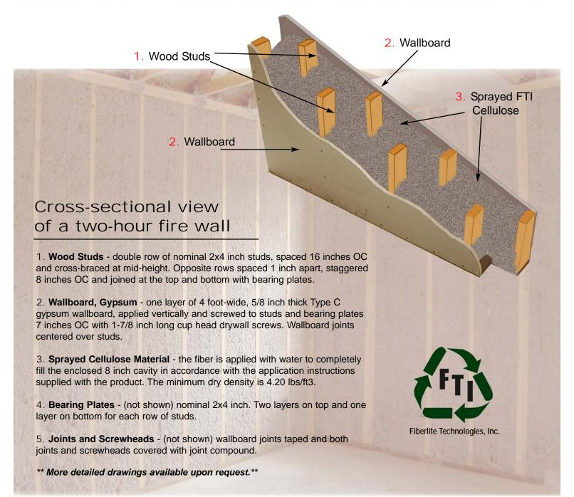
FTI's load-bearing, two-hour fire wall has been tested under ASTM E119-07a "Standard Test Methods for Fire Tests of Building Construction and Materials" by Intertek Testing Services NA, Inc. (Report No. 3132554-1,2 dated November 29, 2007)
